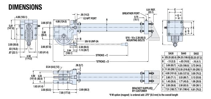
BORE SIZE 4 00 2 50 in 3.00 280 279 280 MAX STROKE 7112 7087 7112 mm MAX **PSI** 200 100 500 **PRESSURE** bar 13.8 6.9 34.5 1248.9 1532.4 MAX FORCE 1398.4 lb OUTPUT 6816
