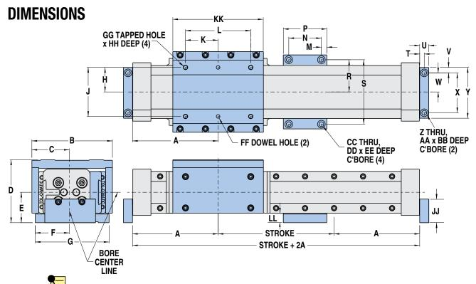
NOTE: In vertical mounting applications, supplemental mounting may be required besides factory foot mounts. Optional Tube Supports and Foot Mounts are shown.
