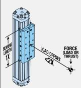
For applications using Solid bearings, binding or interrupted motion may occur if the load offset is equal to or greater than twice the bearing length (1X). LOAD OFFSET is defined as: the distance from the applied force (or the load center of gravity) to the centerline of the carrier.
