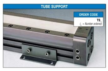
For intermediate support, tube support brackets can be mounted to the BC3 model. Made of black-anodized aluminum, the brackets are attached to the bottom and sides of the cylinder tube with rail nuts. The number of tube support brackets required and their placement depends on the overall length of the BC3 model and the load weight being moved and supported. Refer to the tube support data chart below. Note: Switches cannot be mounted on the same face of the actuator as tube supports.
