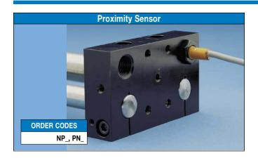
This L.E.D. device senses end-of-stroke with one of two normally open inductive d.c. proximity sensors. NPN supplies a sinking signal; PNP supplies a sourcing signal to a device such as a programmable logic controller.
