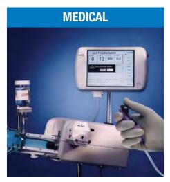
Angiographic-fluid-delivery system combines motion control technology with physician-interactive control.
