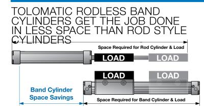
**Consider this:** A rodless band cylinder contains its stroke within the cylinder itself. A 2" bore cylinder with a 24" stroke can provide a 43% space savings when compared to an equivalently sized rod cylinder. In addition, the load is supported throughout the entire stroke so there is minimal load deflection when compared to rod style cylinders.
