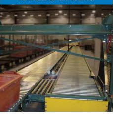
Conveying machinery with built-in lane diverters offer a compact footprint with optimal performance.
