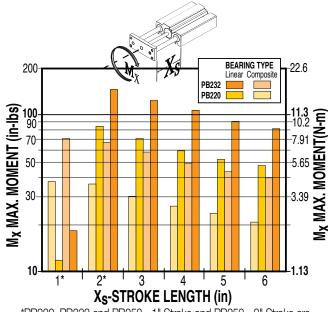
\*PB220, PB232 and PB252 - 1" Stroke and PB252 - 2" Stroke are units with one set of bearings.
