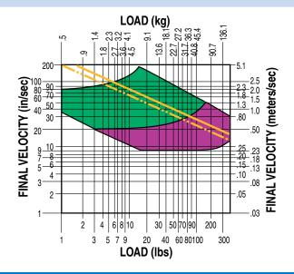
NOTE: If final (or impact) velocity cannot be calculated directly, a reasonable guideline to use is 2 x average velocity.
