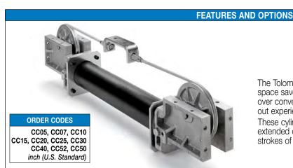
The Tolomatic double-acting cable cylinder is a versatile space saver, available in all 9 bore sizes. Enjoy cost savings over conventional rod cylinders in strokes over four feet with out experiencing rod buckle.
