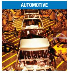
Servo actuators used in resistance spot welding (RSW) increase weld quality.
