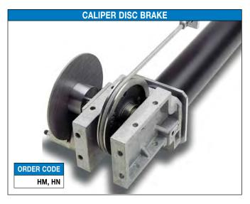
Caliper disc brakes can be used to add holding force in horizontal applications and aid in deceleration at the end of stroke. Caliper disc brakes must be used with an automatic tensioner to function properly. See page CC 32 for selection information and braking formulae.
